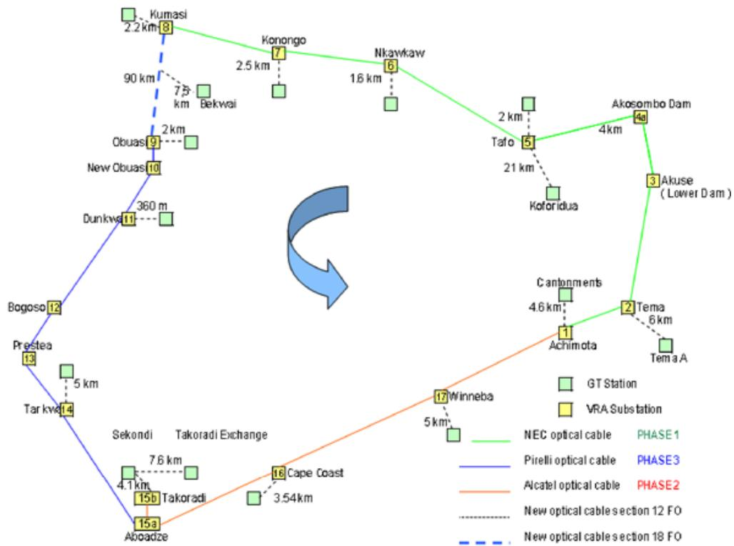
Figure 2: Ghana Telecom and VRA fibre networks
