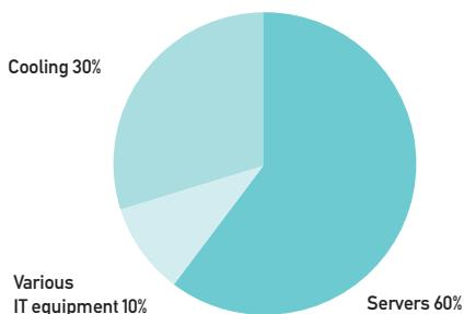
Figure 5: The distribution of electricity consumption in a server room.
