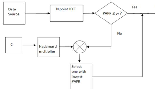
Figure 4: Block Diagram of Selected TR with a Threshold
