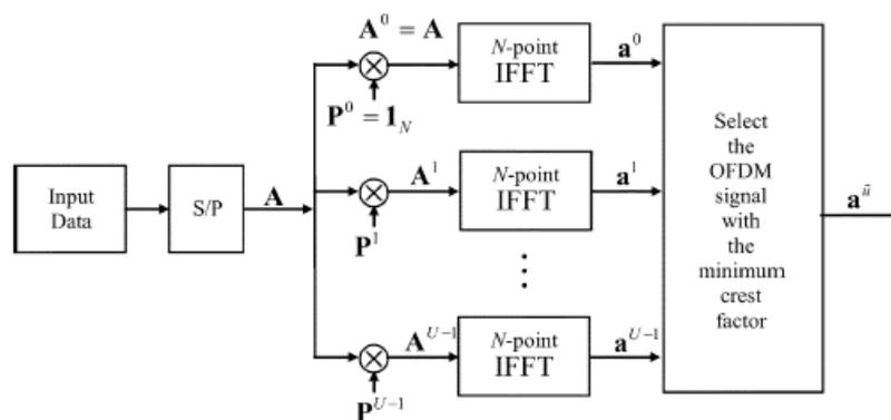
Figure 3: Block Diagram of the SLM OFDM Scheme [13]
